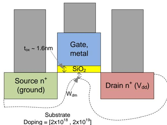
Figure 5 - Transistor Layout, Side View
