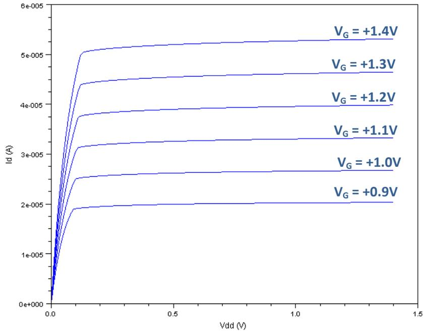
Figure 7 - Plot of  $I_D$  vs  $V_{DD}$  curves,  $W = 32nm$ ,  $V_T = 0.4V$ ,  $V_G = 0.9V$  to  $1.4V$
