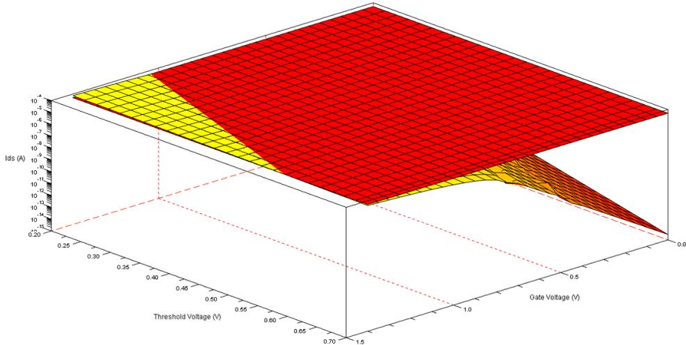
Figure 9 - Plot of  $I_D$  vs  $V_G/V_T$ , for  $V_D = 1.4V$ ; Solution Space Satisfying  $I_{D,min} = 49\mu A$  Highlighted Yellow
