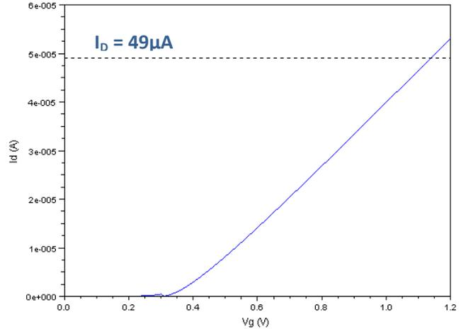
Figure 13 -  $I_D$  vs  $V_G$  Characteristics,  $V_{DD} = +1.2V$
