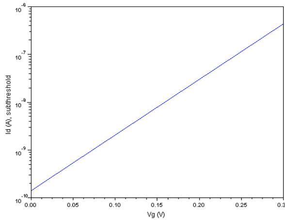
Figure 14 -  $I_D$  vs  $V_G$  Characteristics, Sub-Threshold Region of Operation ( $V_{DD} = +1.2V$ )
