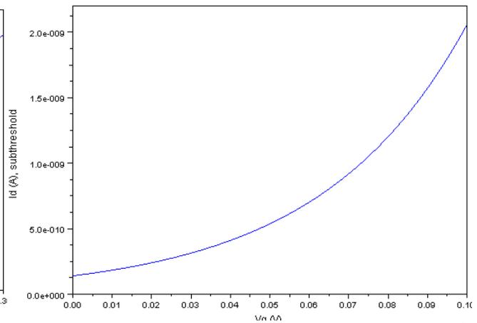
Figure 15 -  $I_D$  vs  $V_G$  Characteristics, Deep Sub-Threshold Region of Operation ( $V_{DD} = +1.2V$ )
