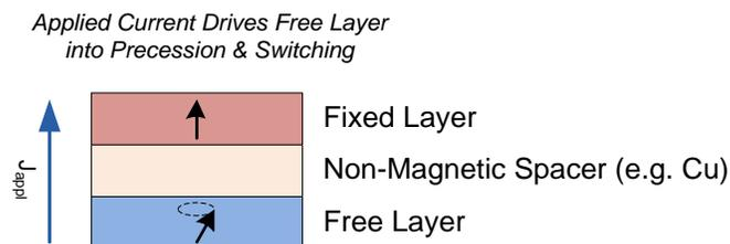
Figure 2 - Schematic Illustration of Applied Current Switching Magnetization in MTJ Element
