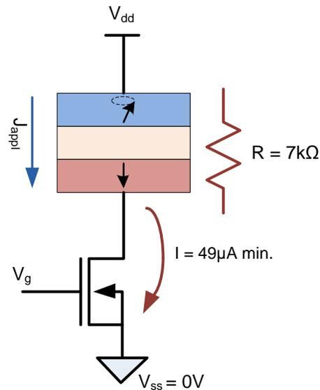
Figure 3 - Equivalent Circuit with MTJ Represented as Series Resistance
