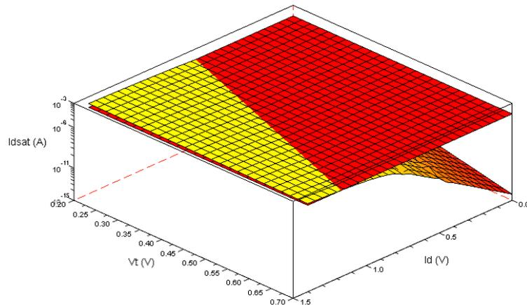
Figure 16 - Solution Space for  $I_{\text{DSAT}} > 49\mu\text{A}$  assuming strain-induced mobility gain of 1.6x
