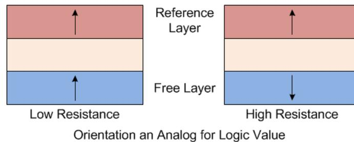
Figure 1 - Schematic Illustration of MTJ Orientations and Corresponding Logic Values
