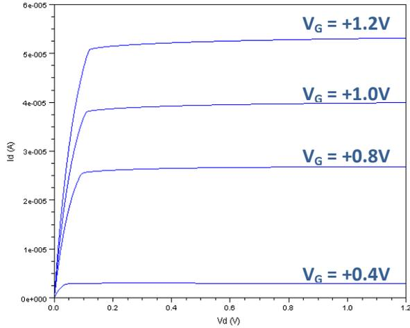
Figure 12 -  $I_D$  vs  $V_D$  Characteristics
