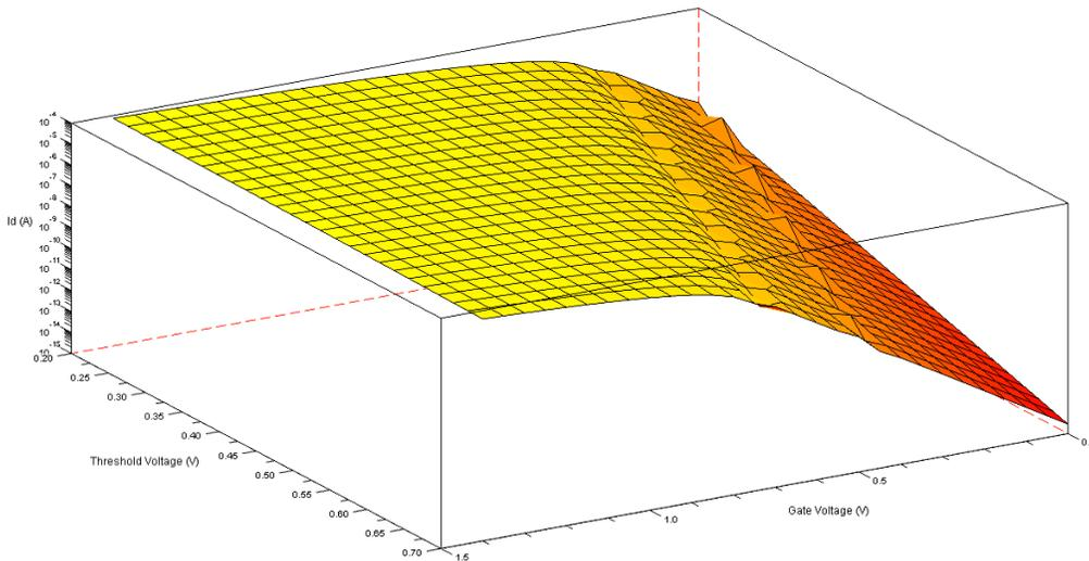
Figure 8 - Plot of  $I_D$  vs  $V_G/V_T$ , for  $V_D = 1.4V$
