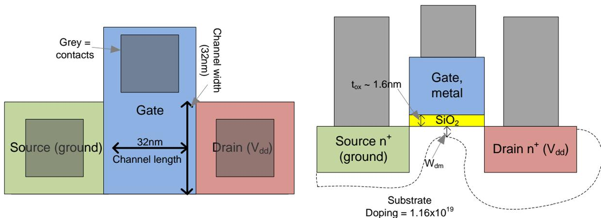
Figure 10 - Final Transistor Layout, Overhead View
